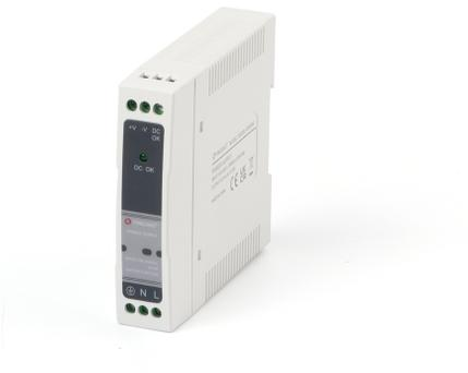
Yingjiao's slimline power family are designed with slim plastic housing and for full range AC input from 90V AC to 264V AC. The series are single phase PSU, providing DC OK relay contact and adjustable DC output voltage. They have high efficiency and operate in wide temperature range. The series can widely used for industrial automation & control systems, varied equipments etc.
