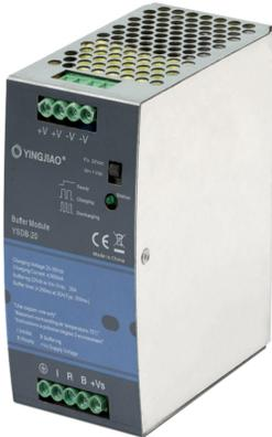
Yingjiao's buffer module is a supplementary device for regulated DC 24V power supplies. The buffer module utilizes maintenance-free electrolytic capacitors to store energy, thus eliminating the need for periodic replacement as compared to costlier batteries which also have shorter functional life span.
